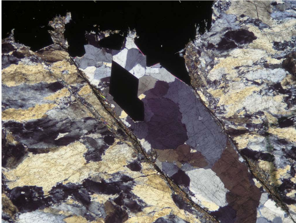
Figure 1: Photomicrograph of sample 1 showing elongate strongly deformed quartz making up the groundmass and weakly to undeformed quartz in a vein with sulphides. XPL, FOV = ~ 7 mm.
